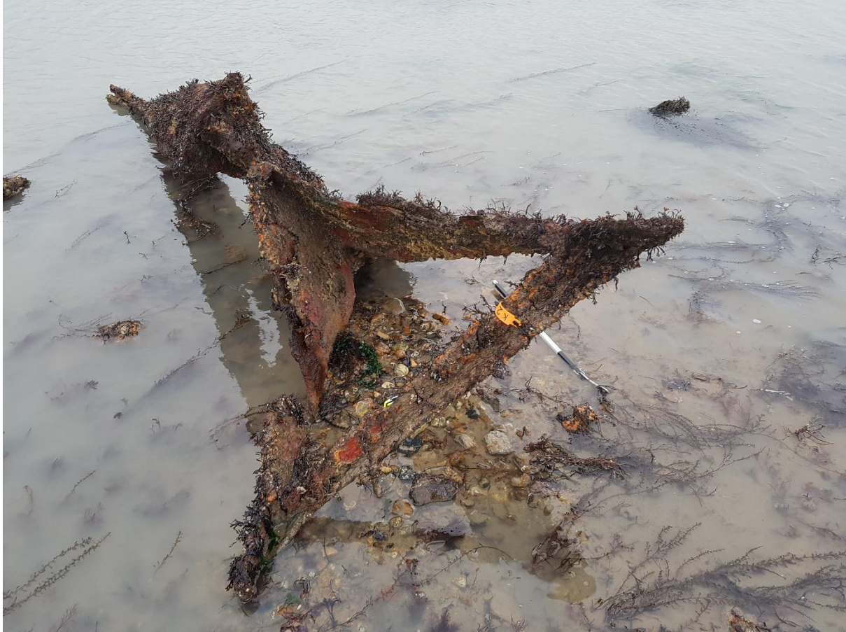
Figure 14. Kite Anchor K2 in shallow water showing the corrosion to the hook plates.
