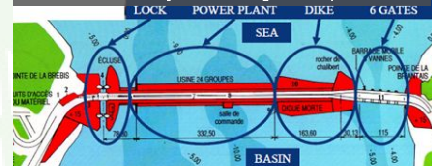
The Rance Layout showing the Ship Lock
