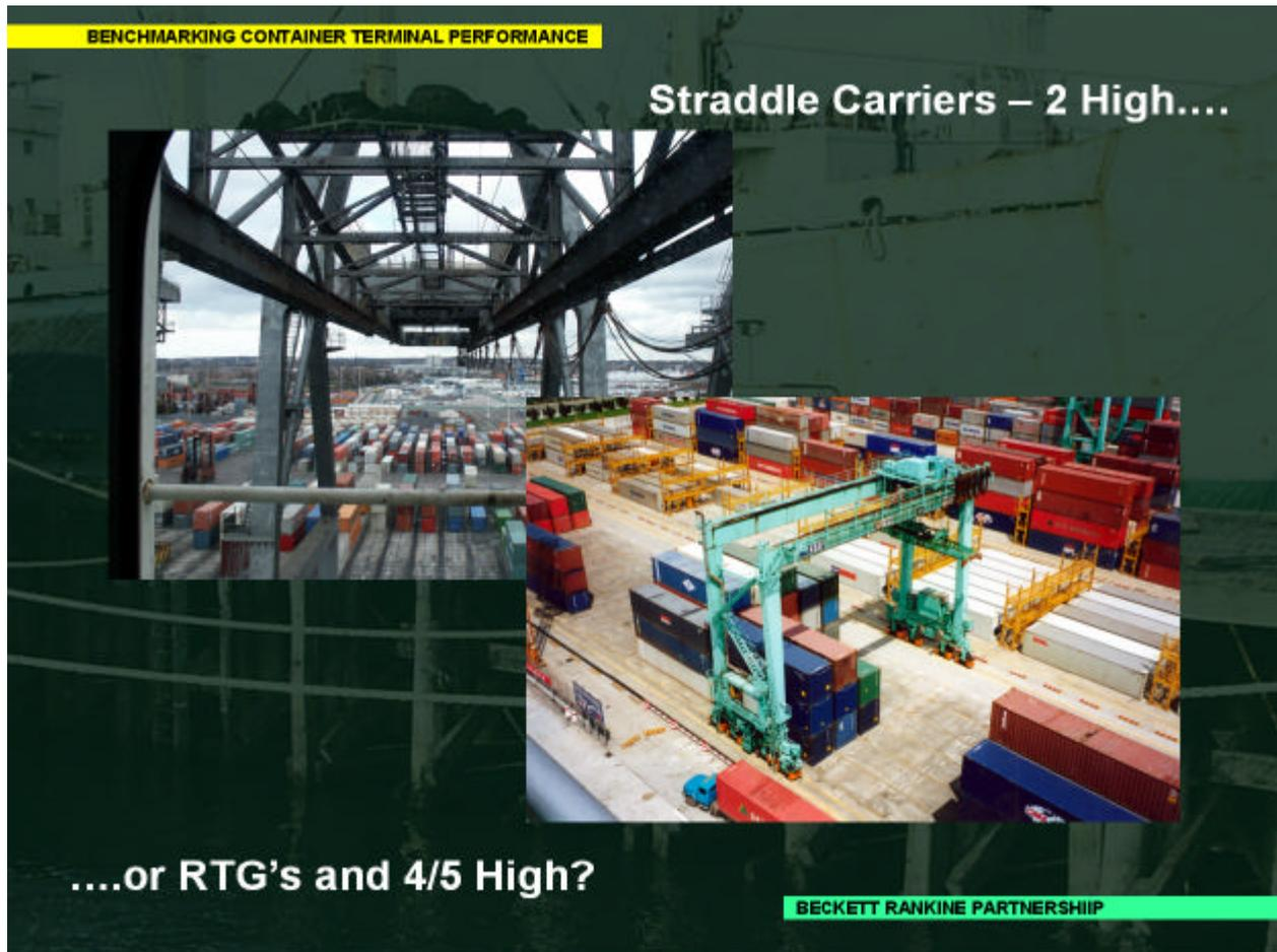
Clearly terminals using straddle carrier operation with large areas and low stack heights will show a low utilisation. This does not necessarily mean that they are inefficient, but it could be that large areas of land are readily available and, in any event, there is a substantial potential for growth.
